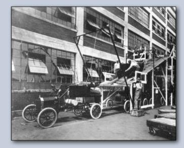
1913 Experimenting with mounting body on Model T chassis. Ford tested various assembly methods to optimize the procedures before permanently installing the equipment. The actual assembly line used an overhead crane to mount the body.
